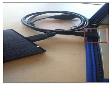
Connect the USB connector (it said SS on the top of the USB connector) into the USB port
